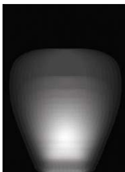
Light distribution elliptical T12° x L44°
