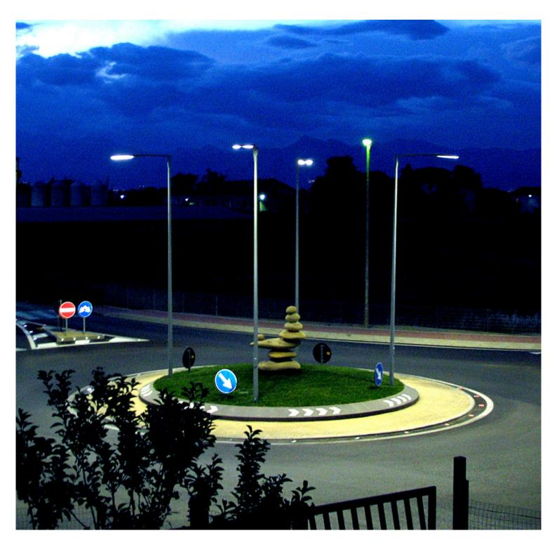
With StyLED now in place, the maintained average luminance had been improved to a fully compliant 37 lux with good uniformity and glare control
